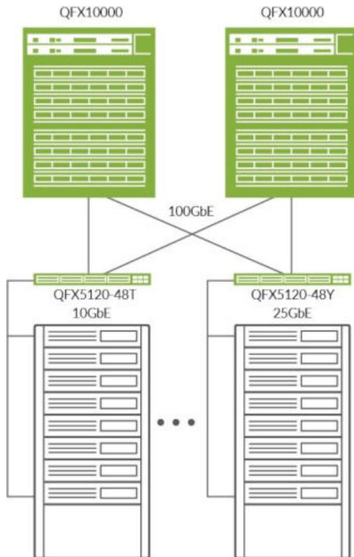
Figure 3: QFX5120-48Y and QFX5120-48T in a leaf-and-spine deployment
